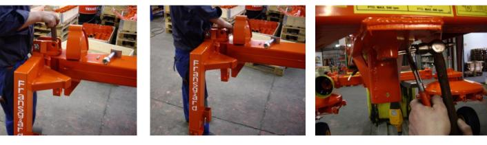
Step 7: Fitting the top link attachment
