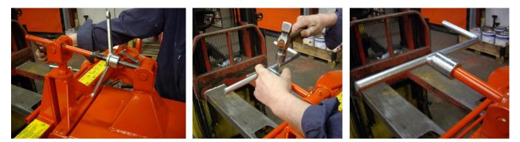
Step 6: Fitting 3-point hitch to the frame. Remember the roll pin.
