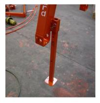
Step 9: Fit the shaft bracket to the frame and the cover for the PTO
