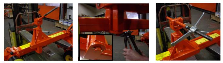
Step 4: Mounting the frame between the rotors and 3 point hitch. Make sure pin rolls are properly mounted
