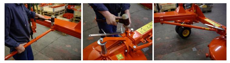
Step 11: mounting safety guard bracket. Important: remember the rubber sleeves Attention: there is a left and right side. Left side is for the swath collector (see step 13)
