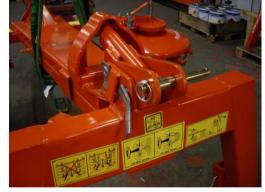
Step 8: fit the brackets for lifting arms. Please be aware of left and right side. Afterwards fit the support leg.
