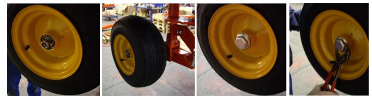
Step 3: Mounting the pivot bracket on to the rotor frame. Do not forget to mount the contra nut
