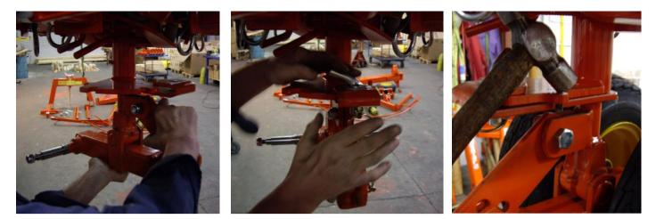
Step 2: Mounting the wheels. Remember tightening nut and dust cap
