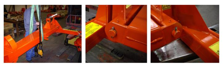
Step 5: Fit the thread rod into the block. Afterwards mount the handle for adjustment.
