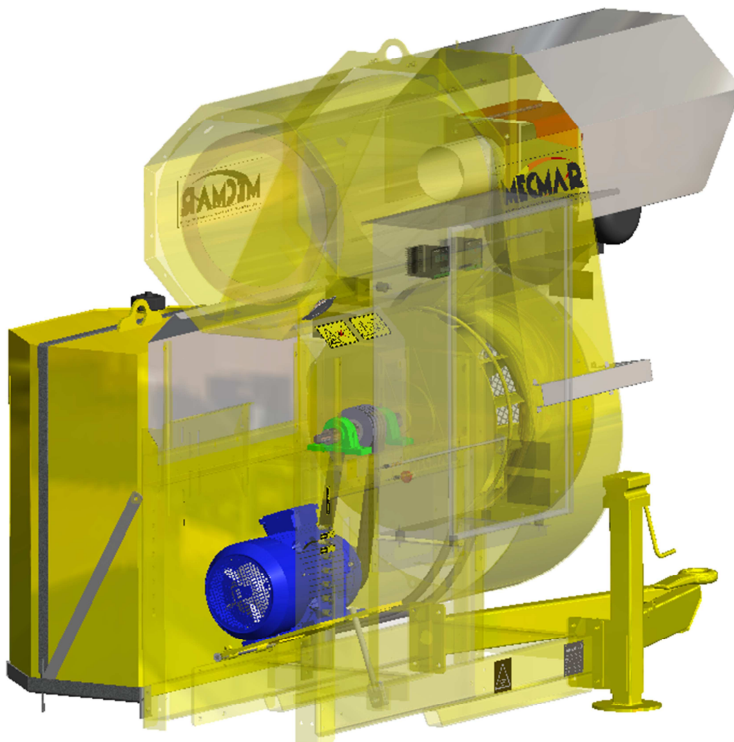
Testata elettrica – Electric transmission
