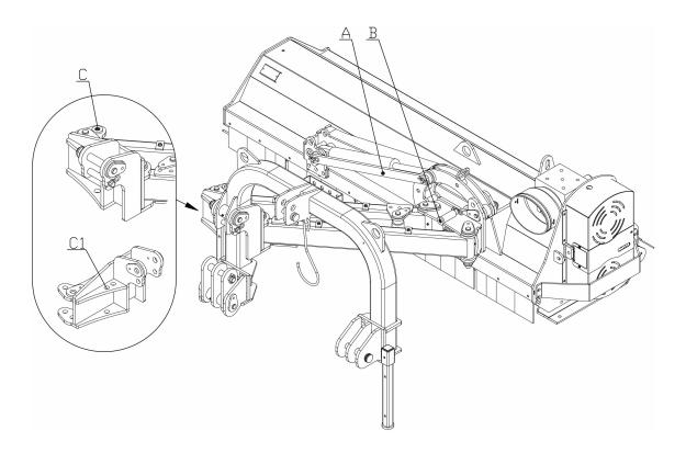
According to the needs of the customer, it is possible to adjust the speed of the hydraulic cylinder of both the side-shifting and rotating system, with the regulator mounted on the connection between the hydraulic tube and the bottom plate of each cylinder.
