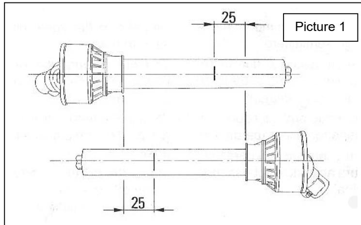
1. Through the hydraulic lift, bring the machine at the minimum distance from the tractor.
