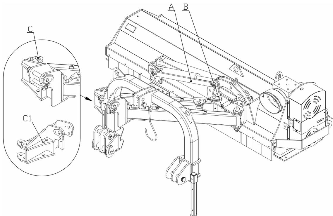
According to the needs of the customer, it is possible to adjust the speed of the hydraulic cylinder of both the side-shifting and rotating system, with the regulator mounted on the connection between the hydraulic tube and the bottom plate of each cylinder.
