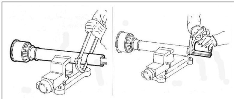
1. Cut the plastic tube with a hacksaw on the line you previously marked on one of the semi-cardan.
