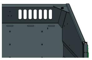
It is easy to see inside bucket by the help of holes in buckets upper back wall and evaluate buckets fulfilment during work.
