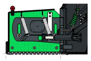
Side wings can be placed on curb stones. They move up 145 mm. That makes collecting of snow easier from narrow streets with sidewalks. Wing reflectors are in standard and LED lights are optional.
