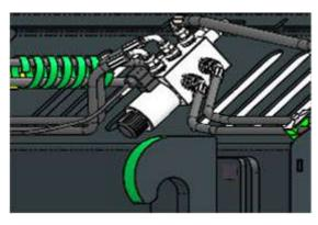
Valve(s) protects the bucket and tractor (or loader) from damage then hitting an obstacle.
